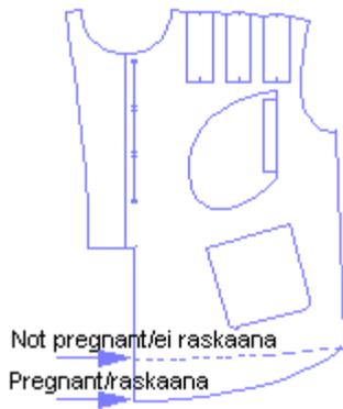
The amount of ease added to the front height is determined by an average value, and may not work in all situations. Therefore, it is important that you check that the **hem is parallel to the floor** all around the garment when fitting the garment on.
